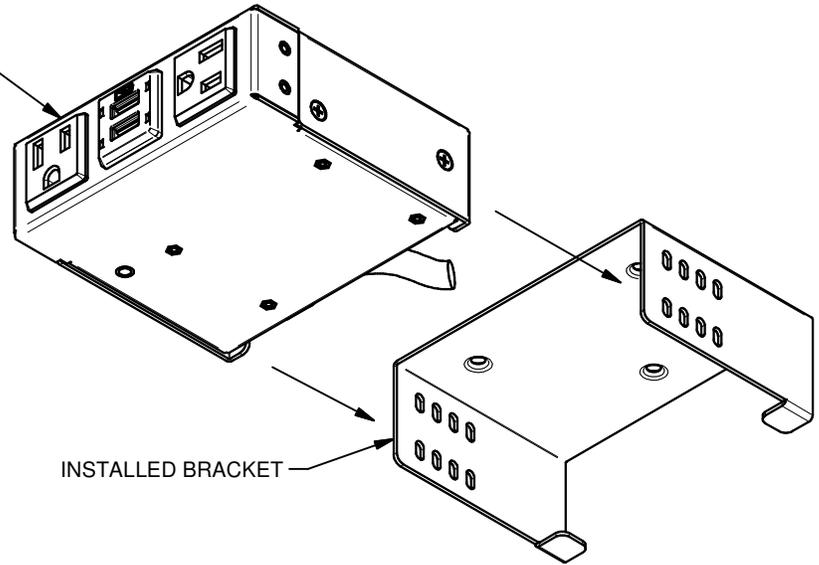
2. SECURE FSR SERIES T6-LB UNIT TO BRACKET AND DETERMINE MOUNTING LOCATION ON TABLE UNDERSIDE.
