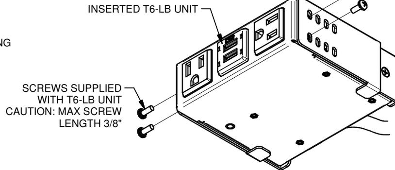
3. REMOVE T6-LB UNIT FROM BRACKET. USE BRACKET AS TEMPLATE FOR PILOT HOLES AND SECURE BRACKET TO TABLE WITH SUPPLIED MOUNTING SCREWS. REINSTALL T6-LB UNIT AND MAKE ELECTRICAL CONNECTIONS AS REQUIRED.
